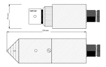
The UCP1B proximity probe is a lightweight and versatile instrument specifically designed to carry out underwater cathodic protection potential measurements.
